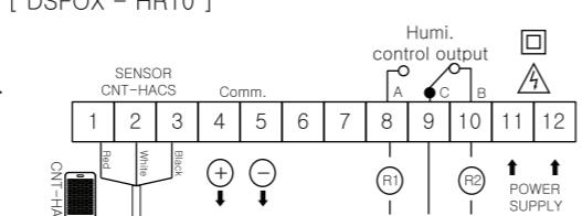
\* Output: 250VAC 2A Be sure to use a power relay or magnet.
