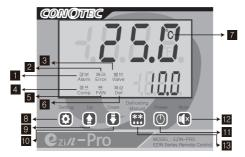
1 Alarm 2 Error indication (inspection request) 3 Electromagnetic valve output 4 Comp output 5 Fan output 6 Defrosting output 7 Display temperature units 8 Setting 9 Up Key 10 Down key 11 Power Key 12 Mute Key 13 Defrosting Manual Key
