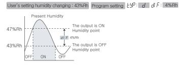
[ A Humidifier → turn off at 43%RH,turn on at 40%RH How to operate(setting for the humidity&programs)? ]
