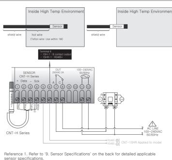
Caution1. A shield wire must be used for sensor wiring, and a high-temperature wire (teflon wire) must be used when used in a high-temperature environment of 65℃ to 80℃.
